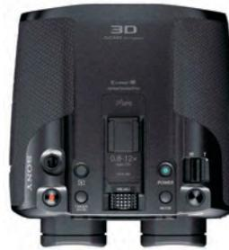
These binoculars zoom from 0.8x to 25x in an instant and they can also record what you're seeing in 3D and keep the picture steady with image stabilization. You can record to several kinds of Sony
